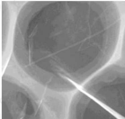
TEM image of Carboxylated graphene
